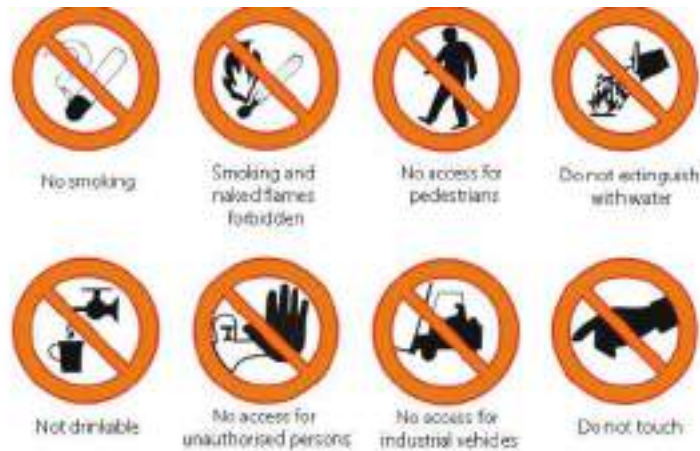
Fig.11.2.8 Safety warning signs
